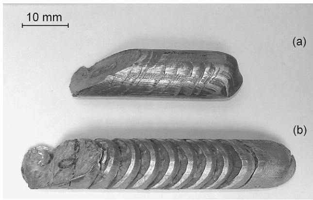
Fig. 7. Samples of Al 7075 alloy, ECAPed after (a) less than 3 min and (b) 10 min of natural aging.
